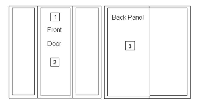
Deflection / Permanent Set was measured with Three (3) Dynavision Laser indicators SN-S1002145, SN-S1002142, and SN-S1002143
